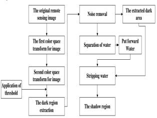
FIGURE 3 Flow chart of shadow detection algorithm
